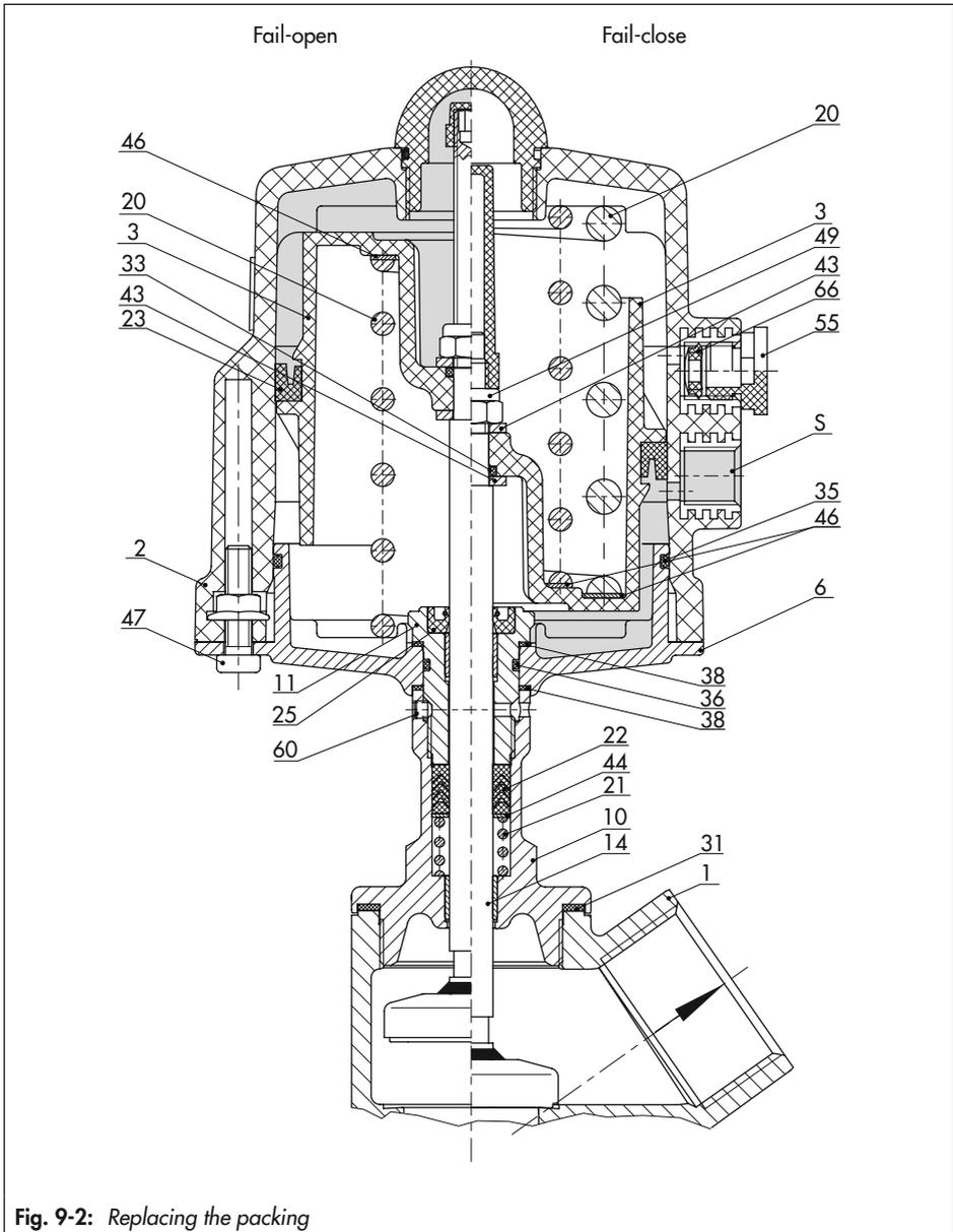
Fig. 9-2: Replacing the packing
