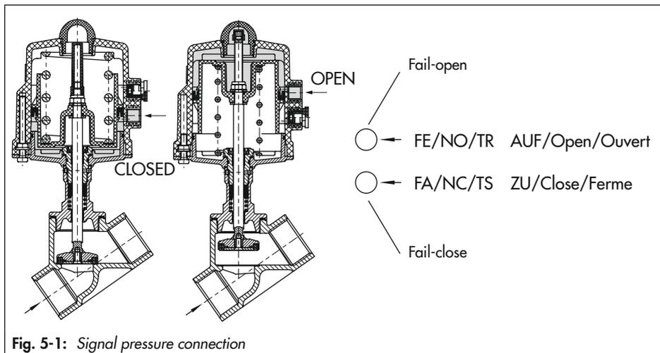
Fig. 5-1: Signal pressure connection
