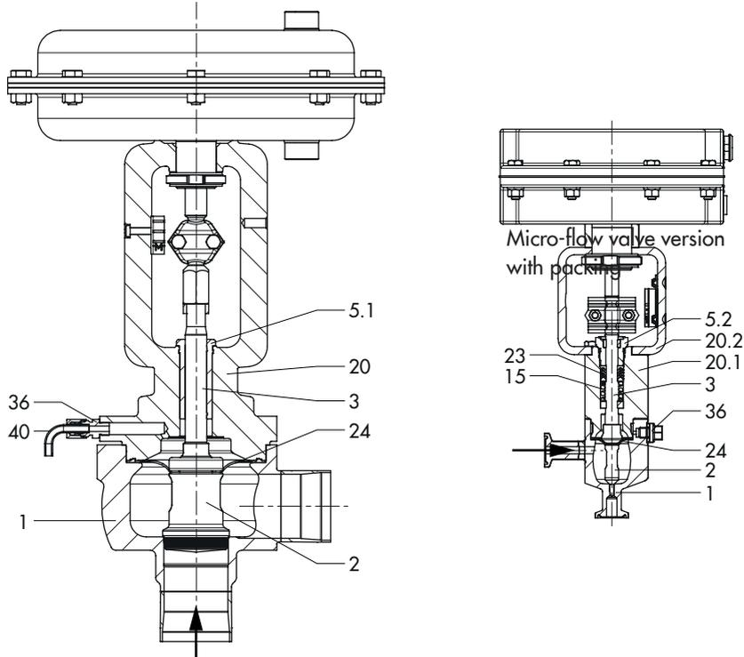
Fig. 9-2: Type 3349 Valve with Type 3271 Pneumatic Actuator
