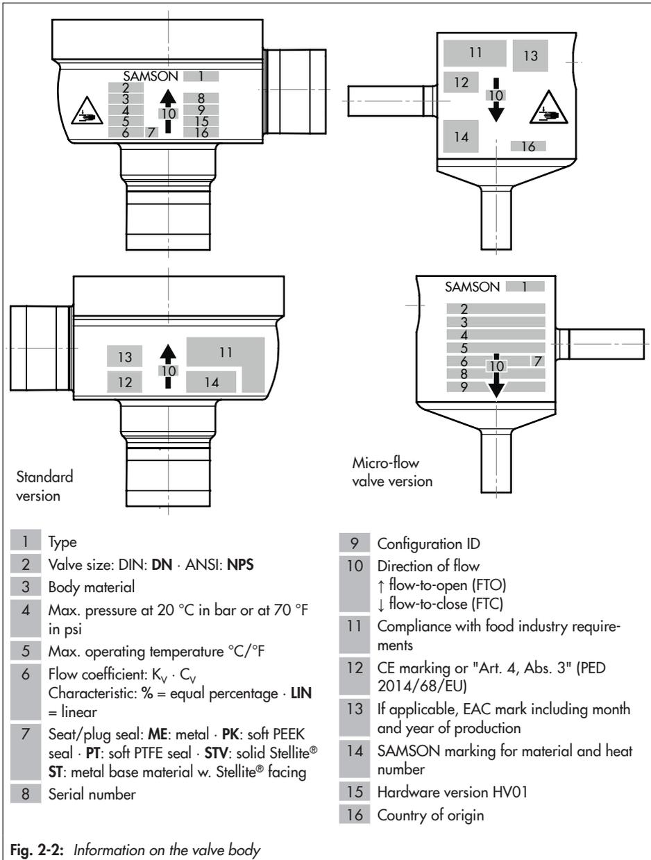
Fig. 2-2: Information on the valve body
