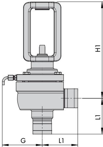
Type 3349 Angle Valve for mounting on
