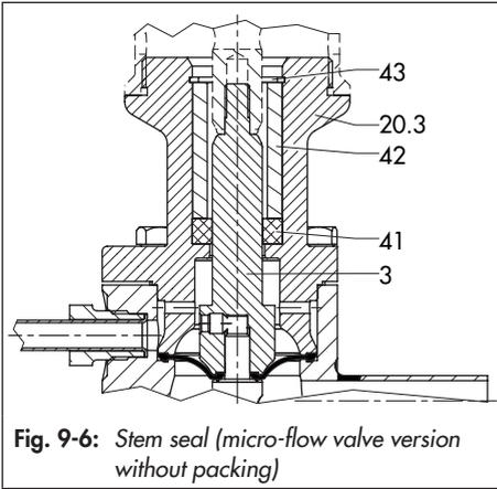
Fig. 9-6: Stem seal (micro-flow valve version without packing)
