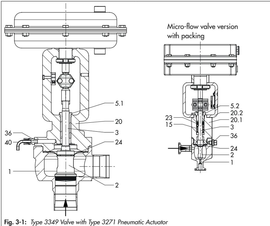
**Fig. 3-1:** Type 3349 Valve with Type 3271 Pneumatic Actuator
