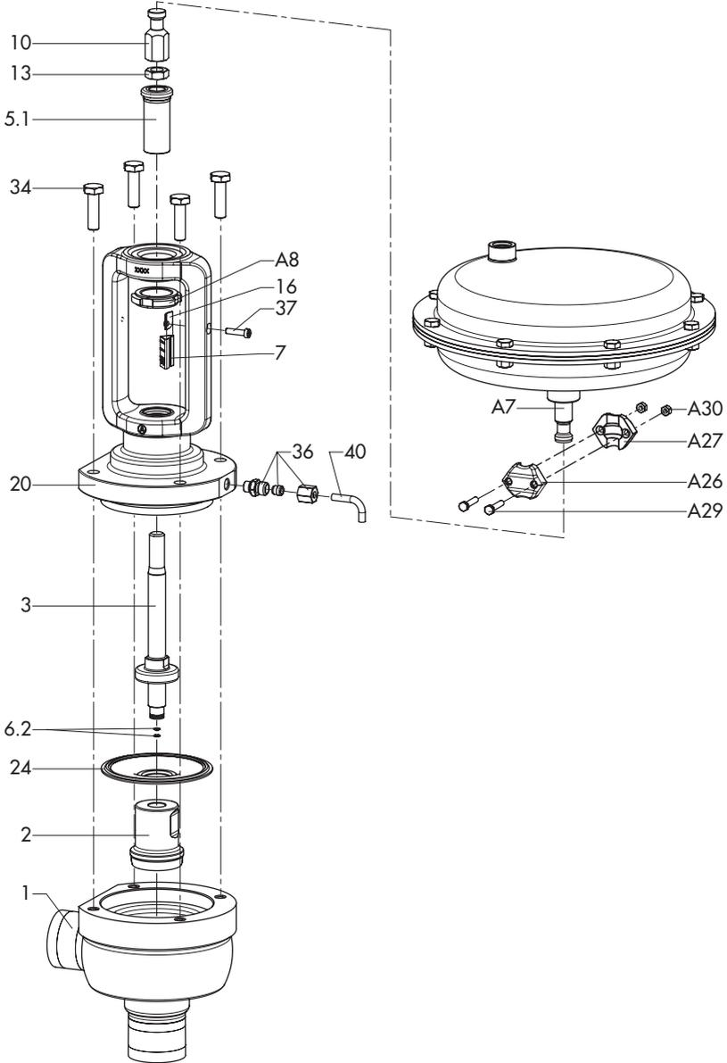
Type 3349 Valve with Type 3271/3277 Actuator - Micro-flow valve version
