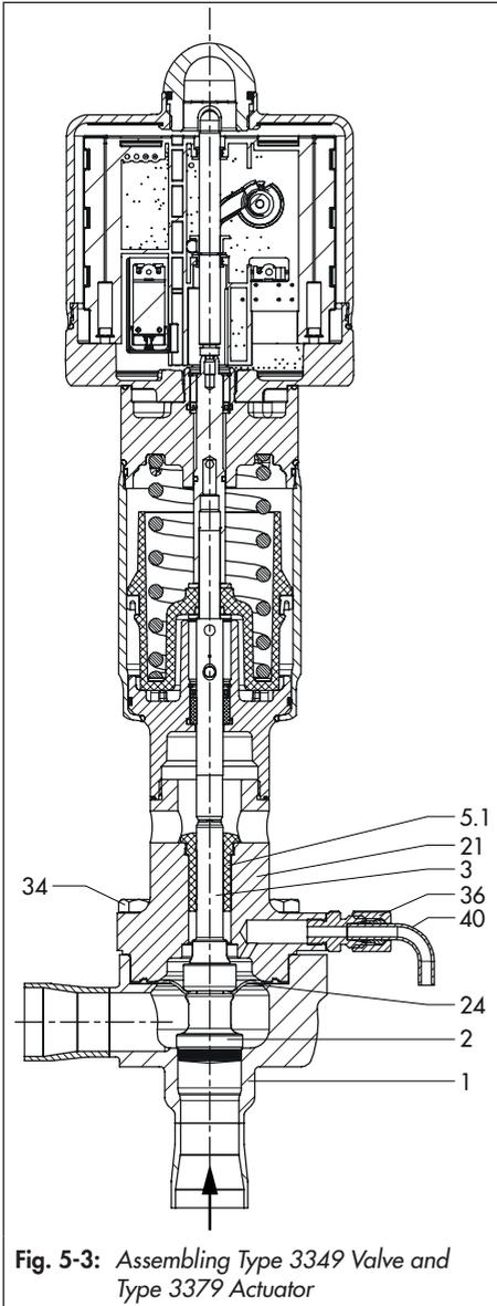
Fig. 5-3: Assembling Type 3349 Valve and Type 3379 Actuator
