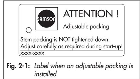
Fig. 2-1: Label when an adjustable packing is installed
