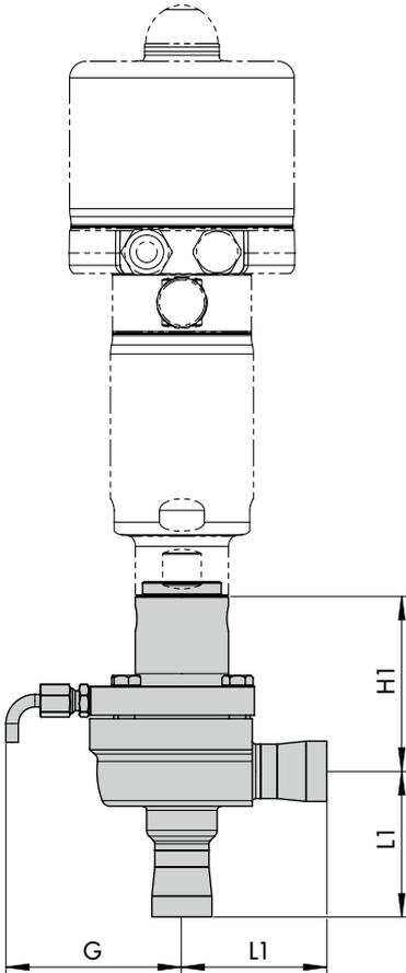
Type 3349 Angle Valve for mounting on Type 3379 Actuator
